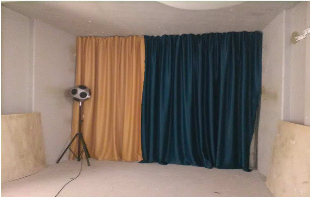
Figura 2_ Reverberation chamber with Sample Configuration 1
