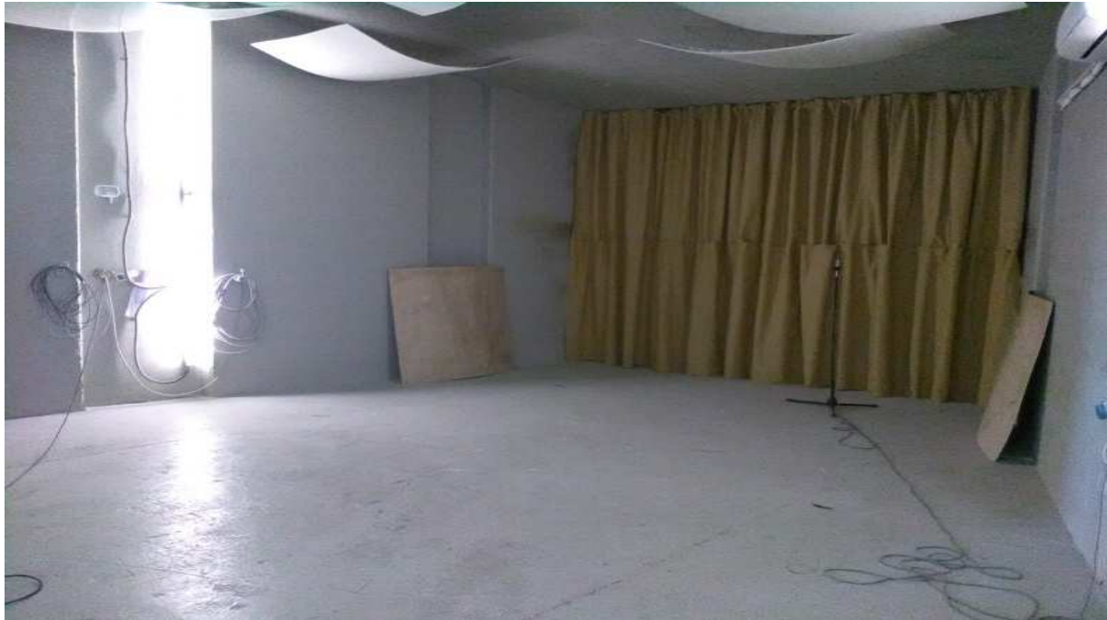
Figura 2_ Reverberation chamber with Sample Configuration 1
