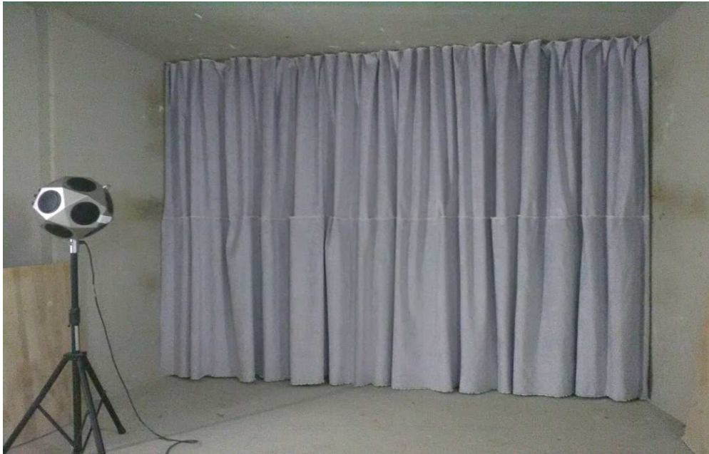
Figura 2_ Reverberation chamber with Sample Configuration 1
