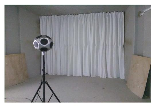
Figura 2\_ Reverberation chamber with Sample Configuration 1
